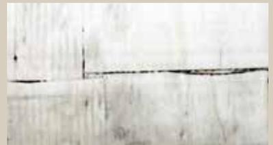
*Photograph of non-structural joints in imported plywood.*
